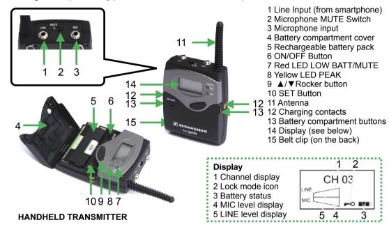
The handheld transmitter is switched on and off by pressing the ON/OFF button on the end for approx 3 seconds. A mute switch is also incorporated.
